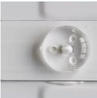
One LED with one PMMA lens
